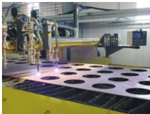
Plasma cutting of web plate and service penetrations
