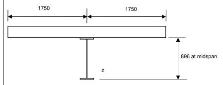
For the effective composite section, taking account of shear lag, the cross girder is effectively simply supported and thus  $L_{\rm e} = 11700$  mm and  $b_{\rm ei} = 11700/8 = 1438$  mm each side. Assume that there is only a single row of connectors on the beam centreline.
