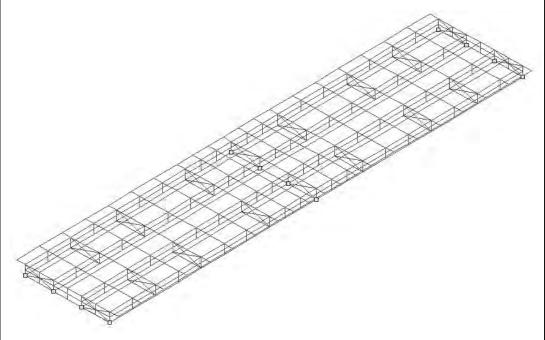
Concrete diaphragms were provided at both abutments, with vertical support only (soil pressures were applied as equal and opposite hydrostatic pressures at the two ends).
