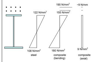
The values at the flanges are at the mid-thickness of the flange
