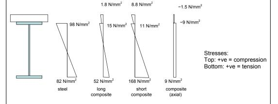
For verification of cross section resistance, the stresses should not exceed the limiting stresses  $f_{yd}$  and  $f_{cd}$ .
