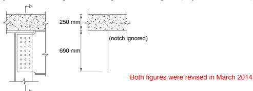
The rules in EN 1994-2 for determining the effective width of the top flange do not cover this situation, where there is an end moment from the warping restraint of the girder, rather than continuity. For the design of the connection it was judged that a width of slab equal to the width of the main girder top flange should be used.
