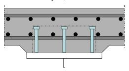
For a critical shear plane around the studs (type b-b in 4-2/Figure 6.15 and shown dotted above) the shear resistance is provided by twice the area of the bottom bars.
