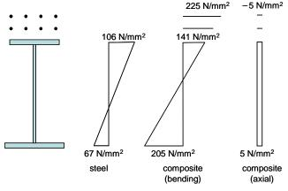
The values at the flanges are at mid-thickness of the flange
