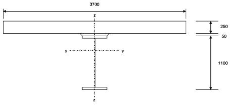
Gross section properties are needed for global analysis. For section analysis, consider the effective section, allowing for shear lag:
