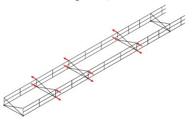
In the model, the forces at the top flange are applied at the model nodes, which are above the level of the steel flange, at the mid-thickness of the slab. The lever arm is thus 1400 - 250/2 - 40/2 = 1255 mm
