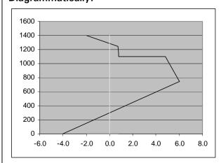
The release of the restraint moments is applied along the span, in the uncracked regions, as a separate loadcase, to determine the secondary effects of vertical temperature difference.
