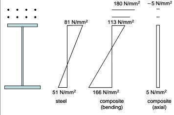
The primary stresses due to shrinkage do not need to be added (see 4-2/7.2.1(4)) and all stresses are less than  $f_y/\gamma_{M,ser}$  (=345 N/mm<sup>2</sup> for top flange, 335 N/mm<sup>2</sup> for bottom flange) and  $k_3 f_{sk}$  (= 0.8 × 500 = 400 MPa).
