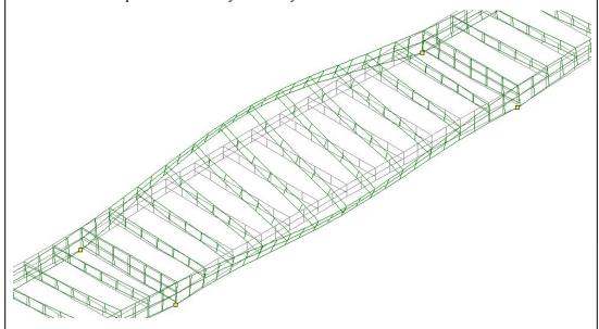
The rotational displacements at the central gross girder, given by the analysis, were  $1.600 \times 10^{-4}$  rad
