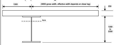
For determination of stresses in the cross section and resistances of the cross section, the effective width of the slab, allowing for shear lag is needed. The following calculations summarize the effective section properties for the sections considered.
