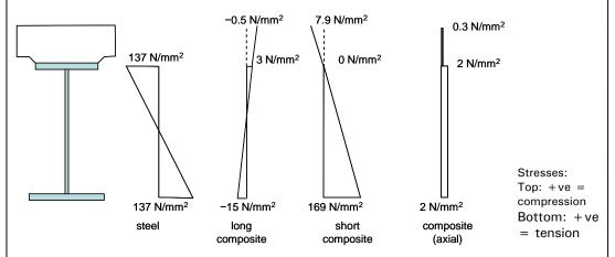
The above stresses include the secondary effects of temperature difference (as an accompanying action). The primary effects should be added (values as an accompanying action): they are 4 N/mm<sup>2</sup> compression at the bottom flange and 1.9 N/mm<sup>2</sup> compression at the top of the slab.
