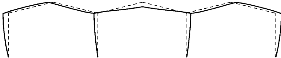
Figure 4.2 Arching failure of rafters
