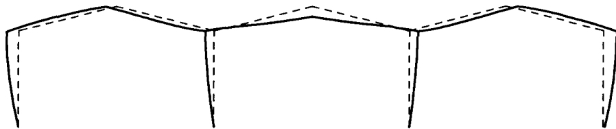
Figure 3.10 Rafter spread in multi-span frames
