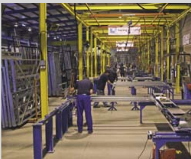
Production of light steel frames. Courtesy, Framing Solutions.
