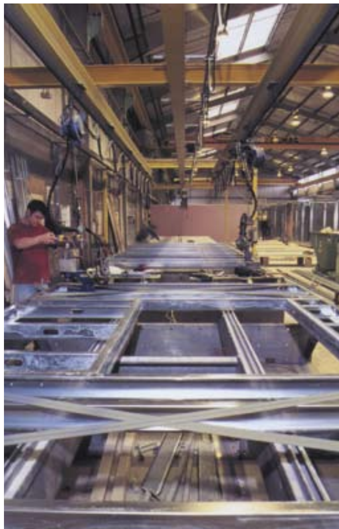
Advanced factory production of light steel framing panels.
