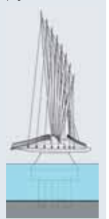
The deck opening mechanism sits on foundations 11m below water level.
