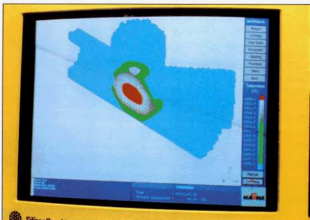
Figure 2.3 Predicted temperature distribution across a section of a steel node during solidification
