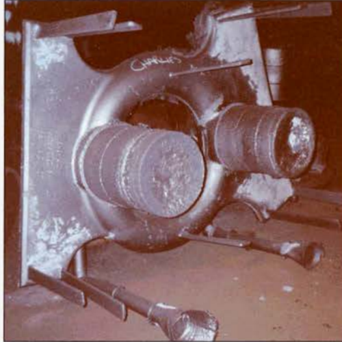
Figure 2.2 Casting for Tees Barrage Bridge just after it was removed from the mould, with risers and feeder heads still attached
