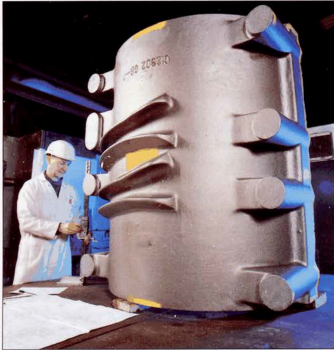
Figure 4.1 Cable band casting for the Tsing Ma Bridge undergoing a dimensional audit
